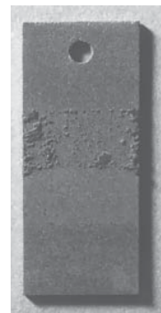
Cement-Metal (CM) One-coat system
